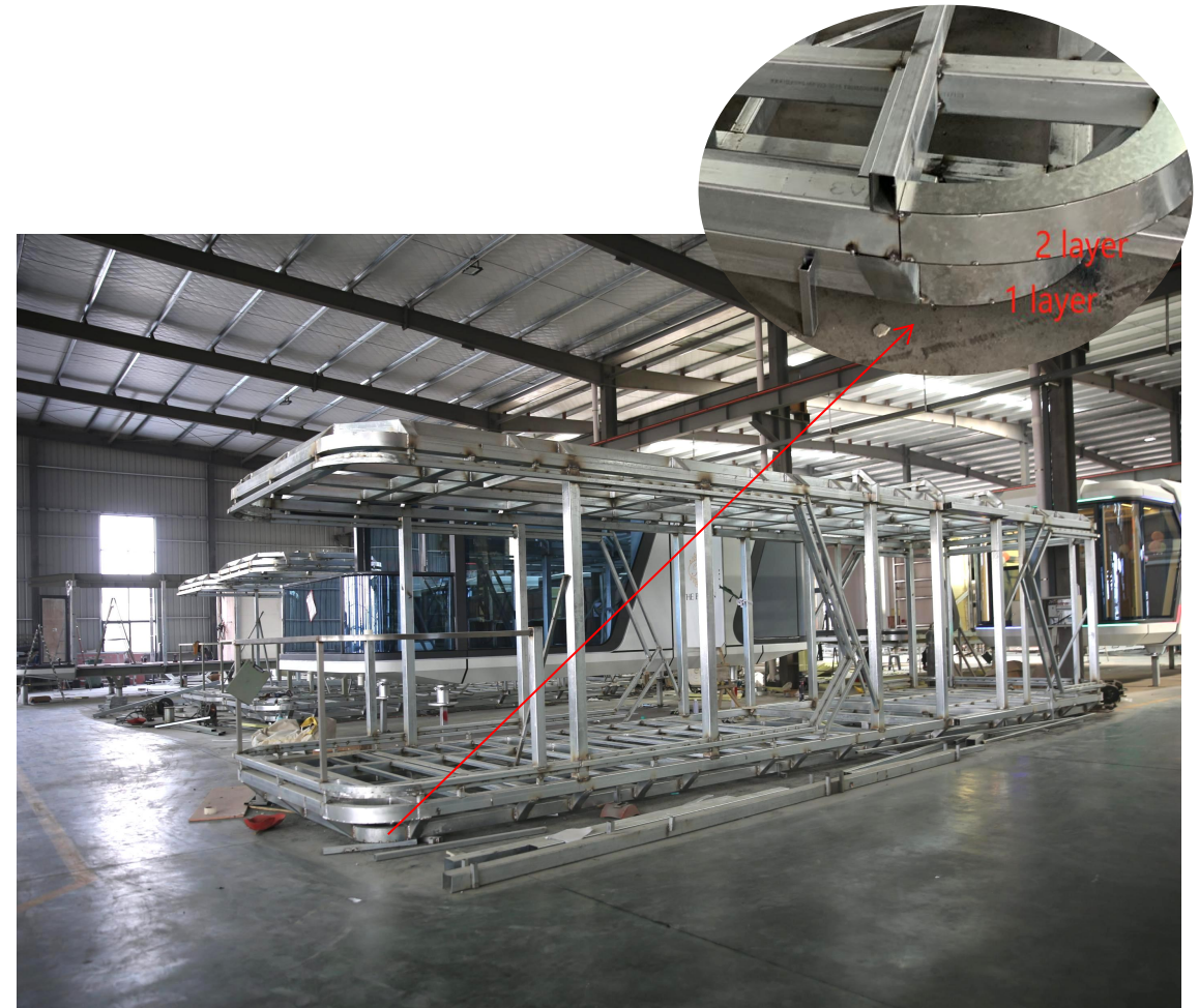
Luban Cabin--The main keel of our capsule adopts 100*100*3 HDG (hot-dip galvanized plates) plate welding, combined with a scientifically arranged framework, to achieve a shock-absorbing effect
